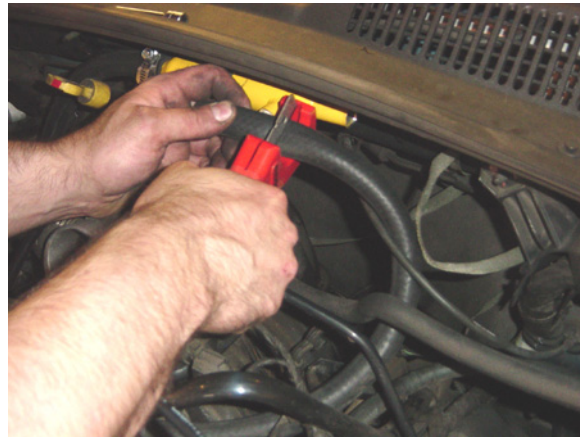
Figure 8 Run a section to the other side, cut, and clamp
