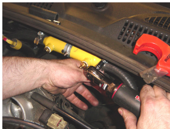
Figure 10 Mounted Cal Cat, tightening clamp
