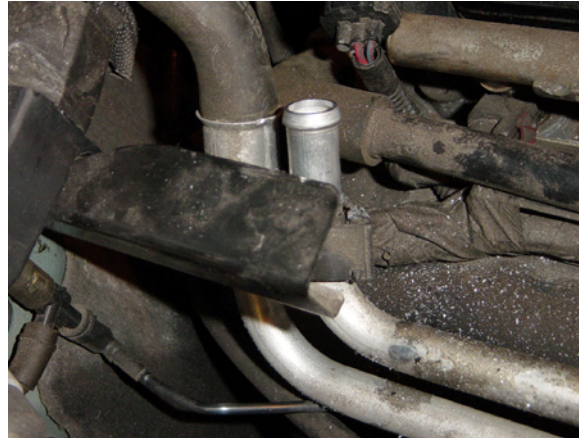
Figure 4 Metal coolant line is bypassed
