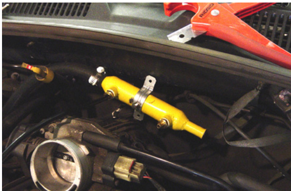
Figure 7 Heater hose attached to the Cal Cat
