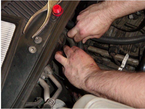
Figure 5 Installing the heater hose
