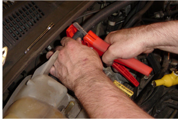
Figure 6 Cut heater hose to length
