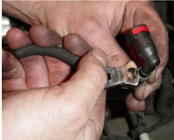
Figure 15 and crimped with the special pliers
