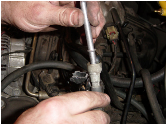
Figure 13 Metal adapter used to connect to stock fuel line
