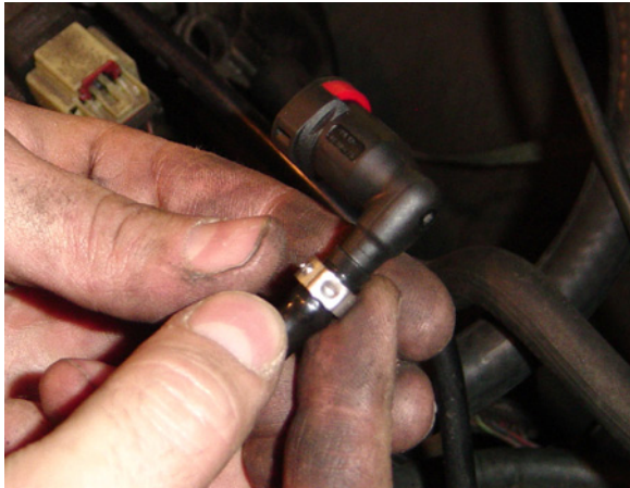
Figure 14 Fuel line is pressed onto fitting with clamp
