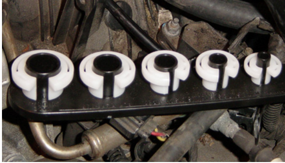
Figure 11 Fuel line disconnect tools
