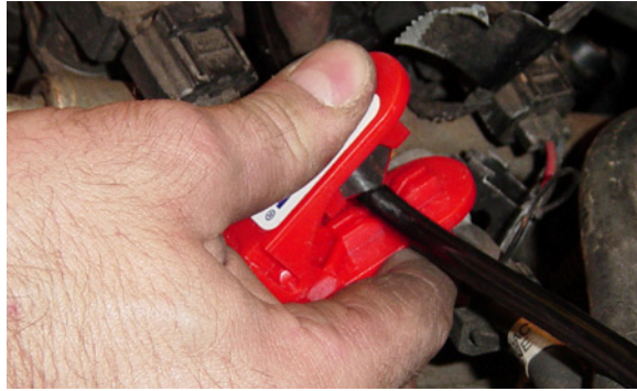
Figure 12 Cutting fuel line
