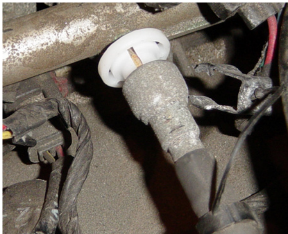
Figure 17 Using the disconnect tool
