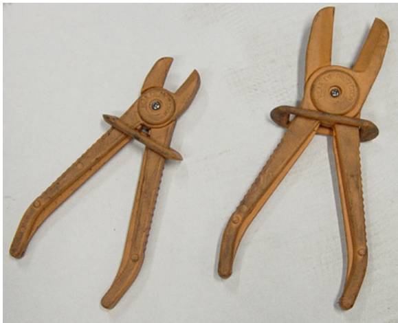
Figure 9 Hose pliers reduce coolant loss
