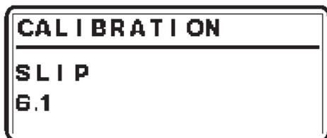
2. Push and hold MULTIFUNCTION button and NEUTRAL button for 5 seconds to enter SLIP CALIBRATION.
