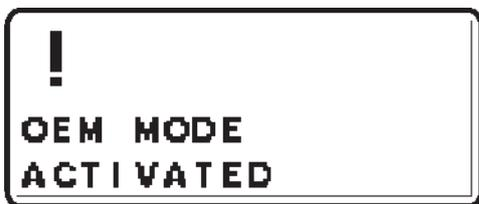
1. Enter OEM-mode by pushing the MULTIFUNCTION BUTTON for at least 5 seconds.
