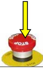
Set Emergency Stop Switch by pushing downward
