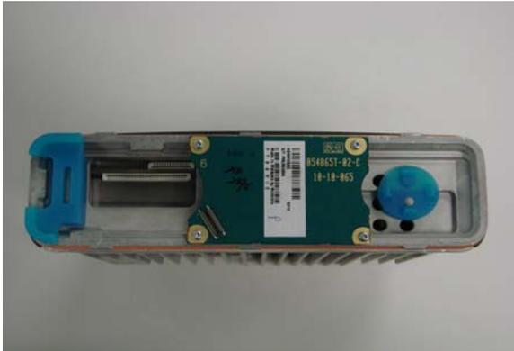
4. Connect one end of the flex cable that came in the HLN7001A option board interface kit, to the small top connector on the radios Printed Circuit Board (PCB) and then connect the control head cable to the large connector on the radios PCB. See the following figure:
