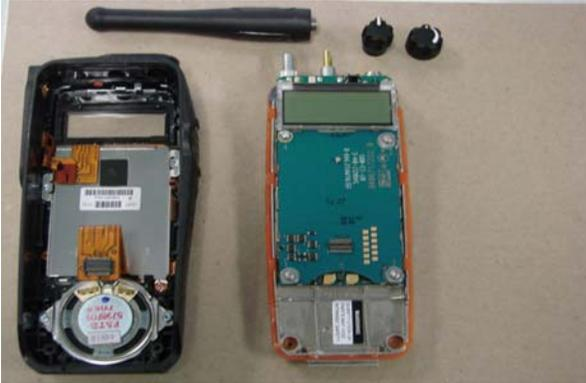
2. Unscrew the four screws securing the Interface Board using a T-6 Torx bit, and remove existing Interface Board 0104022J35. See the following figure:
