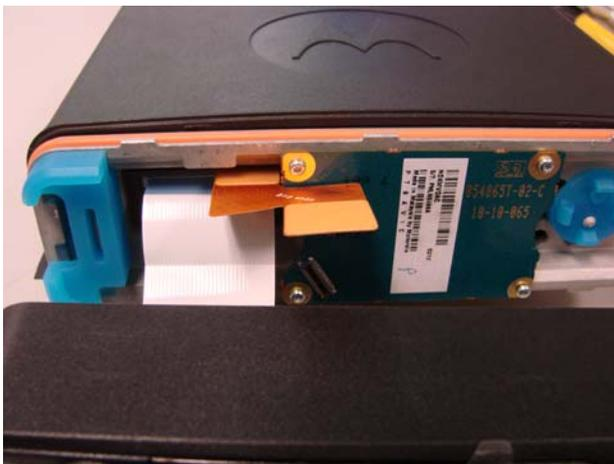
5. Finally, connect the flex cable to the newly installed option board. See the following figure:
