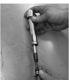
After Dan installs new S&S O-rings into both heads and all four lifter covers, he slips the new S&S adjustable pushrods into their tubes. These pushrods are all the same length until adjusted.
