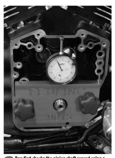
Dan first checks the pinion shaft runout using a dial indicator. He gets only 0.002", which is acceptable. Dan also checked the pinion shaft bushing in the support plate for excessive wear.
