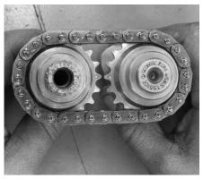
Dan then positions both new S&S cams into the stock H–D inner cam chain with their alignment dots next to each other, noting the directional mark he made on the chain when he removed it.
