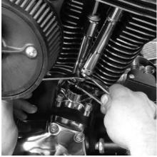
After he has rotated the engine so the front lifters are at their lowest point, Dan positions the front pushrods and tubes in the engine and adjusts them using a 1/4" wrench and two 7/16" wrenches.
