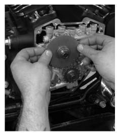
To check that there's endplay on the rear cam, Dan makes sure the rear cam sprocket rotates freely and has slight in-and-out movement.
