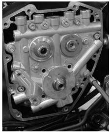
Dan secures the support plate to the right case using the stock bolts, a little blue Loctite, and a 3/16" Allen. He torques the bolts to 90-120 in-lbs. as per the procedure in the H-D manual.
