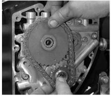
After Dan positions both sprockets into the stock cam chain (noting the directional mark he made earlier) with their alignment dots next to each other, he slips both sprockets onto their respective shafts.
