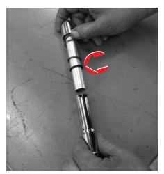
Dan assembles all four S&S pushrod tubes, using the stock collar, spring, and steel washer. The new S&S O-ring is the last part (arrow) on the upper tube.
