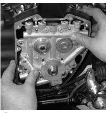
After putting two new O-rings on the right case and putting assembly lube on the cam lobes and chain, Dan slips the support plate assembly into the right case.
