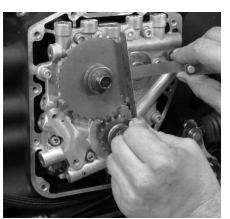
Dan checks sprocket alignment using a steel straightedge across the face of both sprockets. He uses a flat feeler gauge to see that the gap between them is under 0.010".
