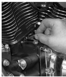
Dan drops the lifters into their bores in the right case with a flat side of the lifter against the wall. He next puts both alignment pins in their slots in the right case.
