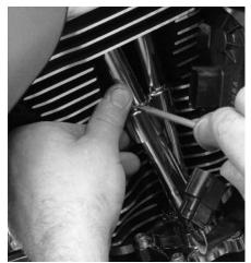
Once the front lifters have bled down and Dan has done the same for the rear pushrods, he pops the top clips into all four pushrod tubes using a flat-bladed screwdriver.
