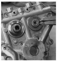
After Dan slips the stock 0.100"-thick spacer over the end of the front cam, he secures it using a new S&S-supplied retaining ring and external ring pliers. He then moves the retaining ring to ensure it's fully in its groove.
