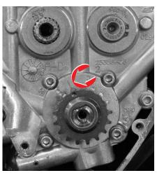
Dan can now remove the rear cam sprocket, and turn the engine over until the pinion sprocket alignment is aligned with the line (arrow) on the face of the support plate.
