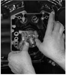
Once he has inspected the oil pump, put some assembly lube onto all the gerotor gears, and slipped a new S&S-supplied 0-ring (don't reuse the old one!) onto the pump snout, Dan reinstalls the pump onto the pinion shaft.
