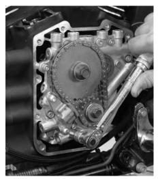
Dan installs the stock outer hydraulic chain tensioner using the stock bolts, some blue Loctite, and a Torx T-27. He then torques the bolts to 90–120 in–lbs.
