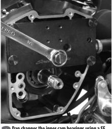
Dan changes the inner cam bearings using a SE puller and installer and the S&S-supplied bearings. Once he has removed the tool, Dan puts some assembly lube onto both bearings.
