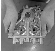
With some assembly lube on the bearing surfaces on the end of the cams, Dan slips the stock support plate over the cams. He then checks that the dots are still aligned using a steel straightedge.
