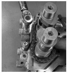
Dan installs the stock inner hydraulic chain tensioner using the stock bolts, blue Loctite, and a 3/16" Allen. He torques the bolts to 90–120 in–lbs.
