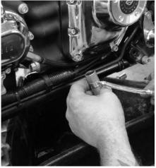
Dan pumps up each of the four new S&S lifters with fresh engine oil through the oil hole in the side of the lifter until the oil comes out of the oil hole in the top of the lifter.
