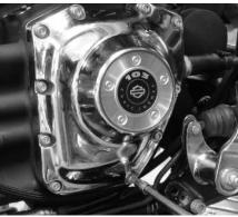
With a new S&S-supplied gasket in place, Dan installs the cam cover using the stock bolts, blue Loctite, and a 3/16" Allen. He torques the bolts to 90-120 in-lbs. as per the service manual procedure.
