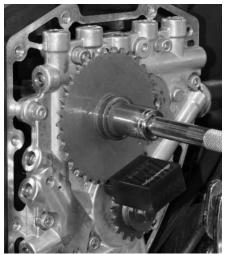
After slipping the original spacer onto the rear cam, Dan secures both stock sprockets onto the rear cam and pinion shaft using the stock hardware, SE sprocket lock, and 9/16" and 1/2" sockets.
