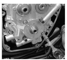
Dan aligns the pump by spinning the engine while using two JIMS alignment dowels, a 5/16" socket, blue Loctite, and the stock bolts. When done, all four bolts are torqued to 90-120 in-lbs.
