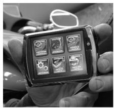
Once Dan has fully assembled the bike and cranked the engine over until the oil light goes out, Rob uses a Dynojet Power Vision fuel tuner and the maps on the S&S web site to dial in the engine. MB
