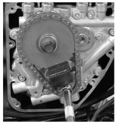
Dan installs the new H-D sprocket bolts and washers using the SE locking tool, red Loctite, and a 1/2" and 9/16" socket. He torques the bolts to 25 and 35 ft-lbs., respectively, as per the service manual procedure.
