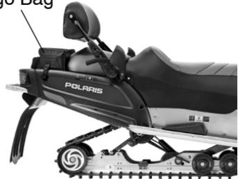
The maximum weight capacity for the cargo area is 30 lbs. (14 kg). Install only accessories specifically approved for this model by Polaris. Always secure cargo before operating. Do not exceed the weight limit. Do not allow a passenger to sit on the seat back or the cargo area.
