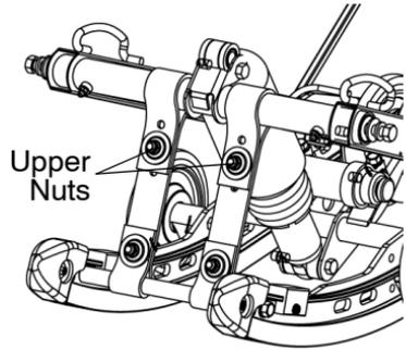
1. Remove the nuts and flat washers from the upper limiter straps.
