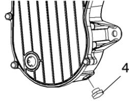
**NOTE:** The sealing surfaces on the drain plug and the oil tank should be clean and free of burrs, nicks or scratches.
