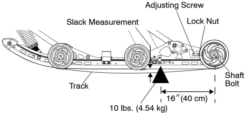
7. Tighten or loosen the track adjusting screws to provide equal adjustment on both sides of the track.
