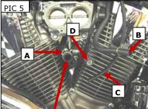
Connect the vacuum line to the nipple on the bottom of the vacuum pod on the back of the Hypercharger with the small hose marked C in PIC.5.
