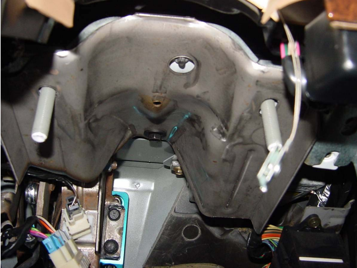
Figure 17 - Modified Cowl Reinforcement Installed
