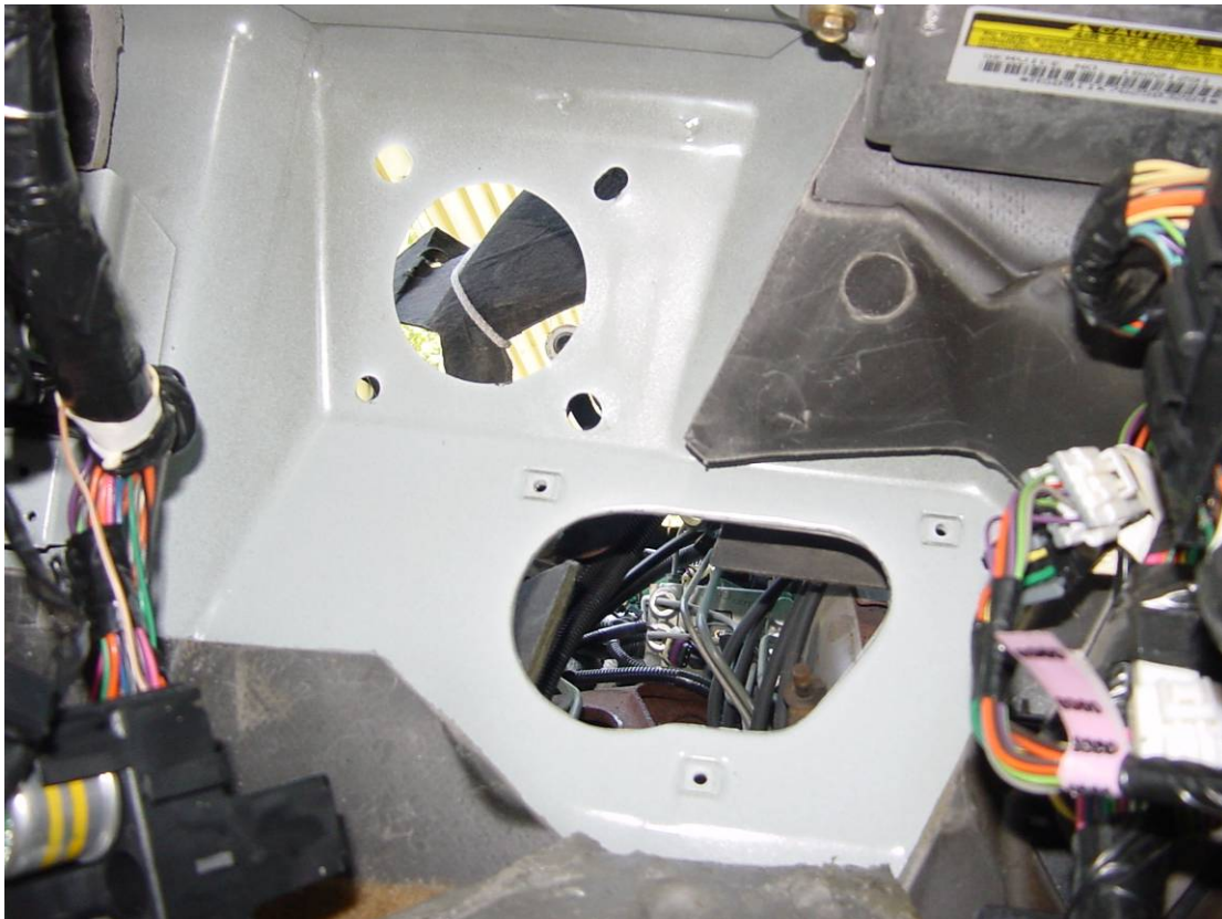
Figure 3 - Firewall with insulation removed
