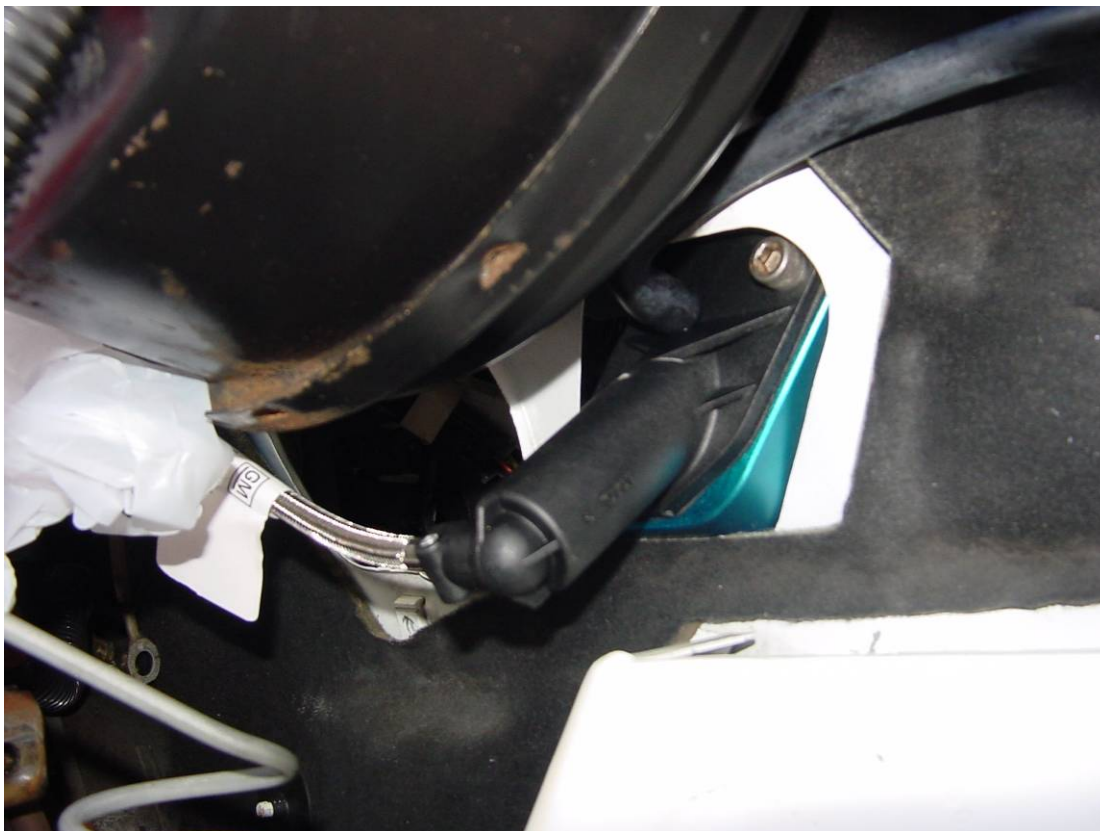
Figure 13 - Clutch master cylinder installed
