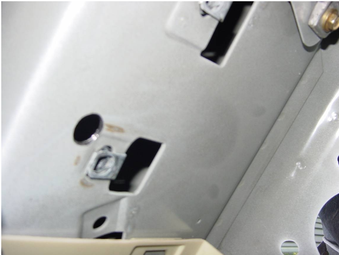
Figure 8 - Completed cowl clearance hole
