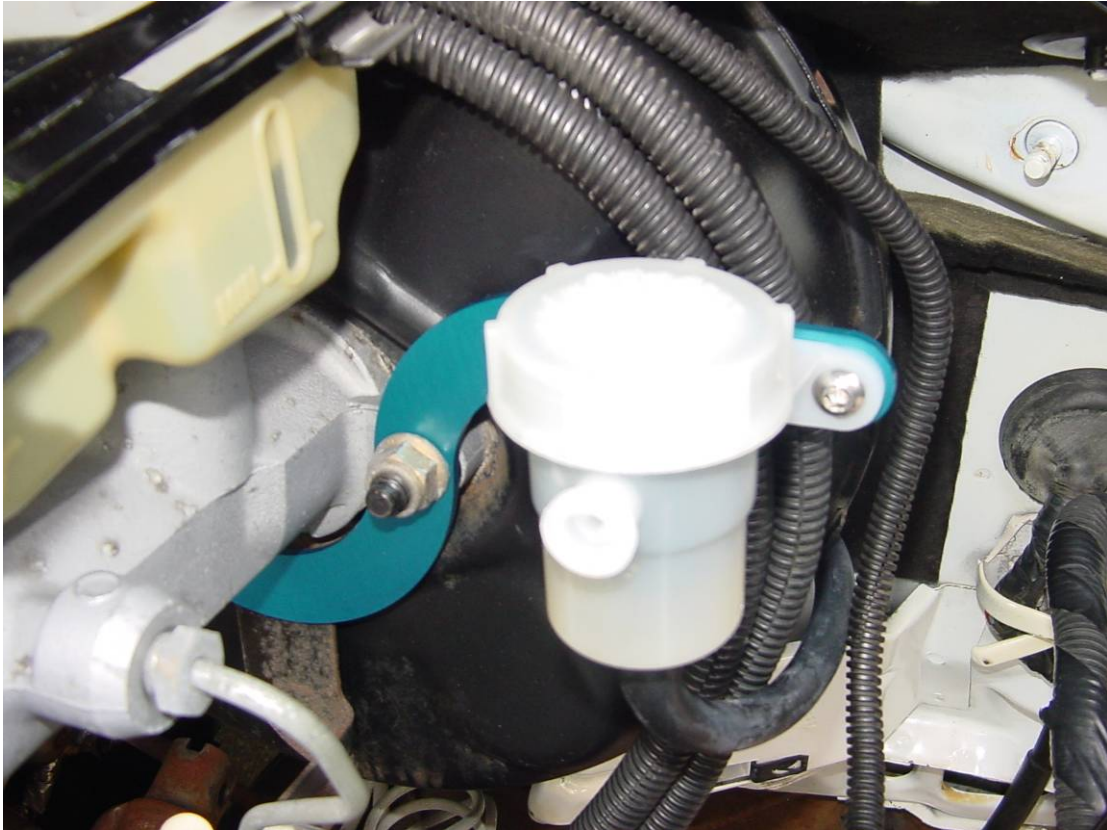
Figure 15 - Clutch fluid reservoir installed
