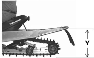
To determine sag, commonly referred to as ride-in, subtract measurement Y from X ( $\text{Sag} = X - Y$ ). Adjust sag by rotating the torsion spring preload cams located on the rear torque arm. See illustration. The ideal amount of sag for this rear suspension is five inches (12.7 cm) ( $X - Y = 5 \text{ in.} / 12.7 \text{ cm}$ ).
