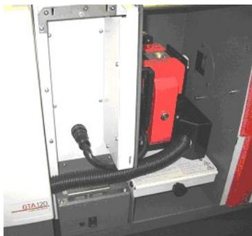
**Figure 5.** Power cable plugged into connector on the 280Z AA
