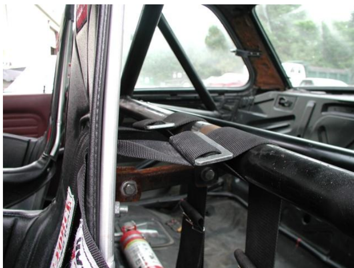
Figure 16. Acceptable Harness Bar and Seat Back Brace Mount.
