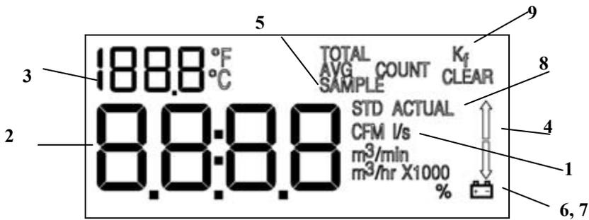
**Figure 3: Display of the Model 8371**
