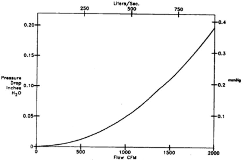
Figure 11: Pressure Drop through the ACCUBALANCE<sup>®</sup> Air Capture Hood
