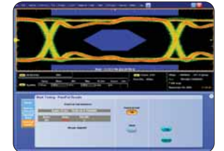
► Testing a 622 Mb/s signal against the mask specified by the standard.
