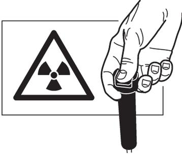
18. Press and hold down the exposure button for the duration of the exposure. The exposure starts when you hear the exposure warning signal and the exposure warning indicator (control panel) and light (side of the unit) come on. The rotating unit will rotate around the patient's head and take the exposure.
