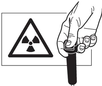
17. Press and hold down the exposure button for the duration of the exposure. The exposure starts when you hear the exposure warning signal and the exposure warning indicator (control panel) and light (side of the unit) come on. The rotating unit will rotate around the patient's head and take the exposure.
