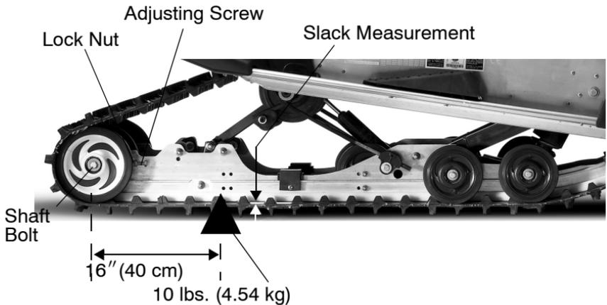
7. Tighten or loosen the track adjusting screws as necessary to provide equal adjustment on both sides of the track.
