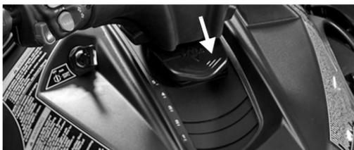
**WARNING!** Do not lubricate the RIDER SELECT mechanism. Doing so could cause loss of control and result in serious injury or death. The RIDER SELECT mechanism is lubricated for life at the factory.
