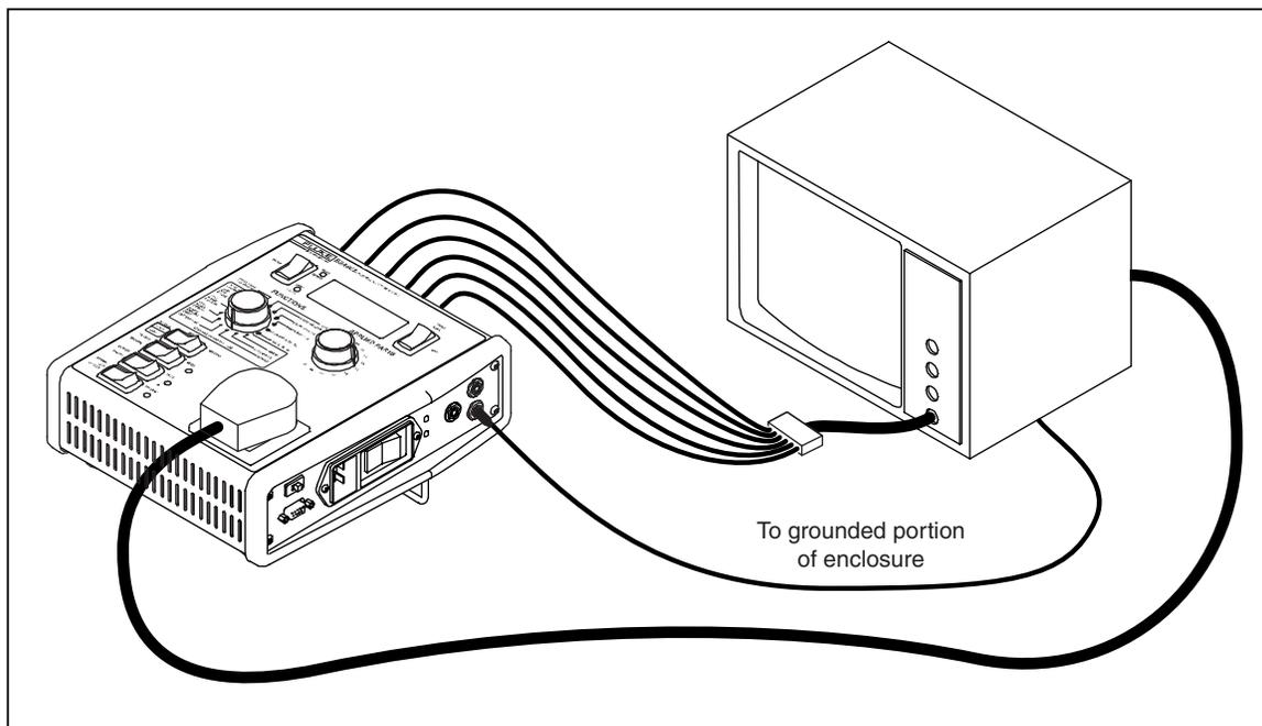
Figure 4-1. ESA601 Connected to a Device Under Test
