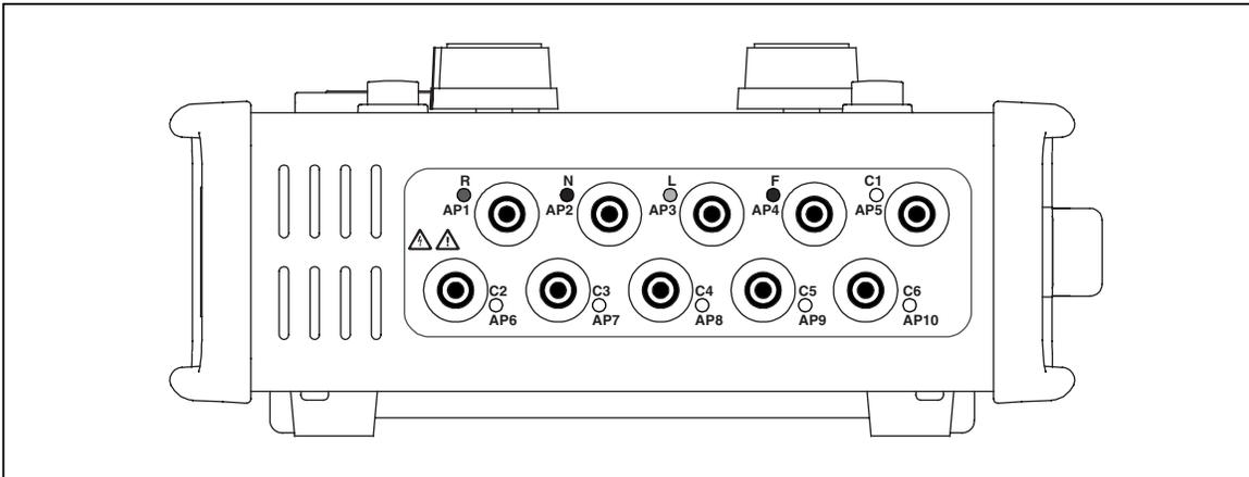
Figure 1-2. Back Panel View of the ESA601 (IEC)
