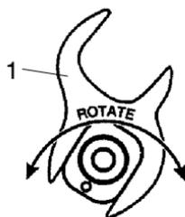
To decrease weight transfer under acceleration (for improved cornering), rotate the RRSS to a higher position.
