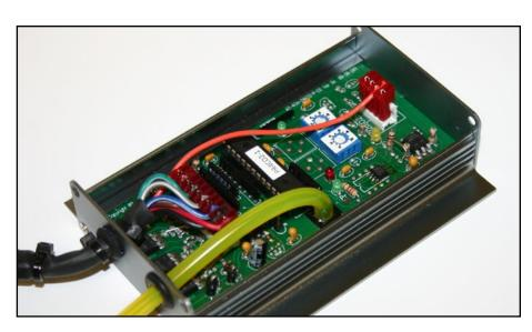
The Voodoo Box intercepts the stock injector signals. When the car is under boost, the signals are modifed to deliver more fuel. Under normal driving conditions - cruise, starting, idling and the like - the injector signal is unchanged. This unit also includes an O2 spoof to eliminate lean tip-in. It does this by modifying the factory O2 sensor under boost while in closed loop.
