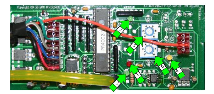
1) The red LED (1) indicates that the board has power. This should be on when the car is on.
