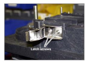
Figure 2-10 Pump band latch
