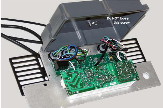
Figure 4-15 Remove power supply cover
