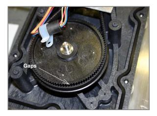
Figure 2-30 Improperly positioned timing belt
