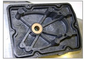
Figure 2-28 Distributor gasket replacement
