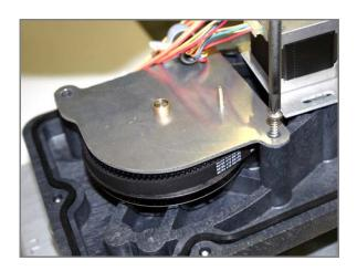
Figure 2-31 Installing the cover plate
