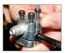
Figure 3-9 Piercing service port .312 O.D. tubing with a saddle tap tool
