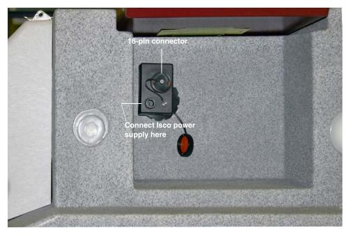
Figure 4-3 5800 battery backup module
