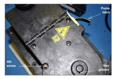
Figure 2-7 Opening the pump housing cover and latch
