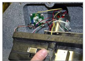
Figure 2-4 Installing the pump module
