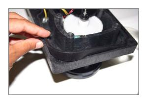
Figure 2-18 Improper installation of pump gasket
