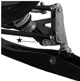
**NOTE:** An excessive adjustment can result in damage to the shock. When adjusting these shocks, we recommend that you turn the screw only 1/4 turn at a time, then test ride.
