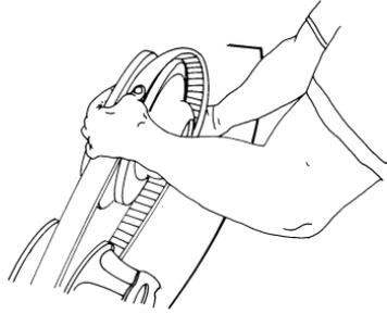
2. Turn the driven clutch moveable sheave clockwise while pushing inward and forcing the belt down between the sheaves.
