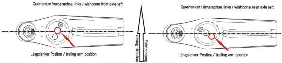
wishbone bearing points may be altered within Stock range of adjustment only.
