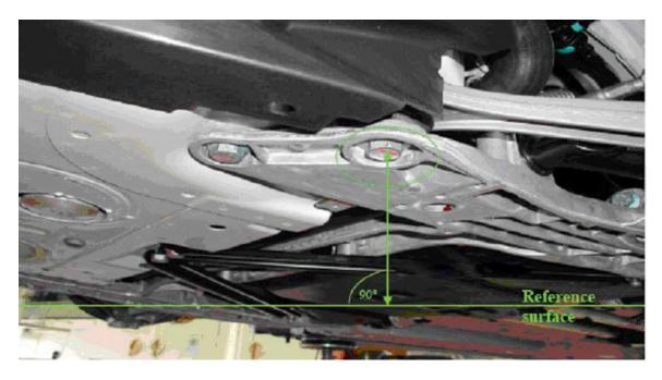
Minimum ground clearance (Ride Height) of rear axle measurement point
