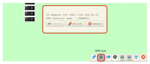
3. Press [Connect] and [Unlink] to change the connection state. A mark appears on the VPN icon in the disconnected state.
