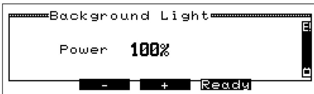
With "▲" (+) or "▼" (-) you may adjust the intensity of the display light. Possible intensity adjustments are: 0 % (shut off), 25 %, 50 %, 75 %, 100 % and Auto (Automatic).
