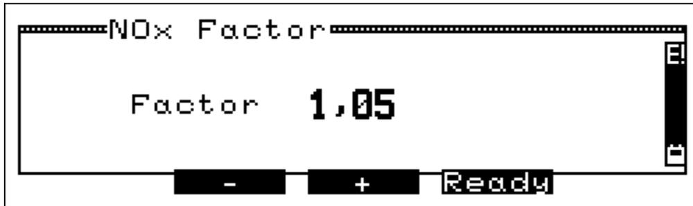
The instrument is able to calculate NOx by taking the NO<sub>2</sub> share of the NOx into account.
