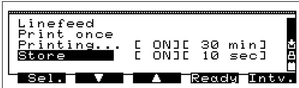
Behind the function “Store” the first brick informs that the automatic storing is switched on or off, the second brick informs about the chosen time interval.
