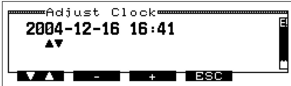
With pushing "ESC" (ESC) the menu "Adjustments" is called again.
