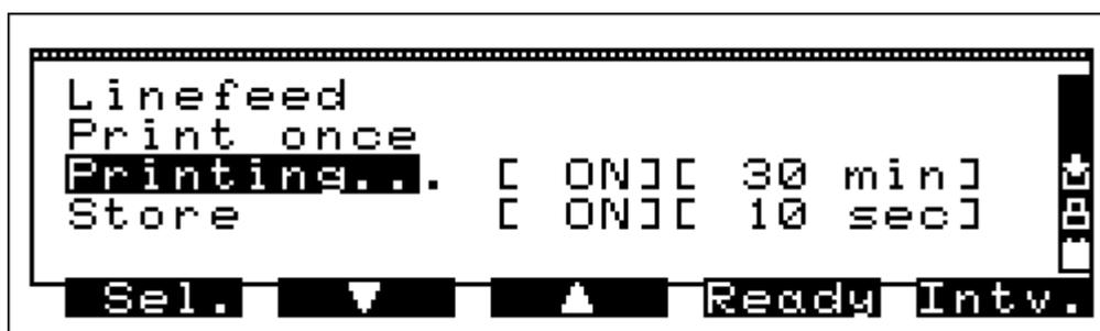
Behind the function "Printing..." the first brick informs that the automatic printing is switched on or off, the second brick informs about the chosen interval.
