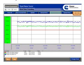
The Touchscreen provides real time trend charts for any monitored value in the system, with up to 8 monitored points at any time. Historical trend charts using a data log function in the control may also be provided (optional). The Historical charts are configurable for functions displayed, and for the time frame displayed, and allow comparison of historical data from multiple time periods simultaneously.
