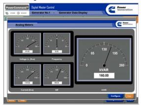
The touchscreen is configurable to AC data in analog "needle type" meter displays.
