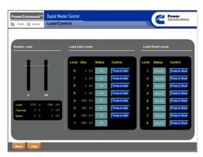
The load control screen provides an analog display of system load as a percent of available capacity of the generator sets that is operating in parallel on the bus. The screen provides an alphanumeric display of this data. It also displays the name, status and priority of each load block (whether on or off), and the total load of that block. The screen allows the operator to manually add and shed loads in any sequence desired.
