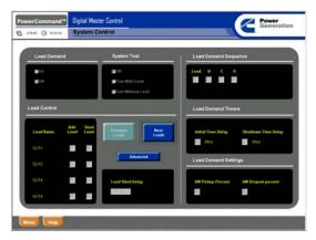
The system control screen provides the operator with the ability to enable or disable load demand operation, view timer values and view the load demand sequence; initiate test (with or without load); control the shutdown sequence for the generator sets in the load demand mode; set the load demand time delays; set the load demand operation set points; and display and modify the automatic load add and shed sequence.
