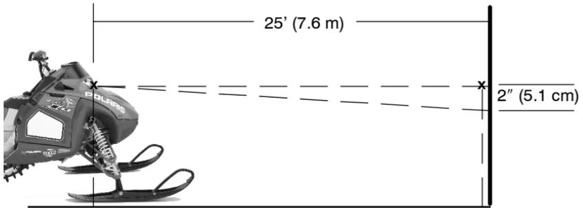
The headlight may be adjusted for vertical aim using the following procedure:
