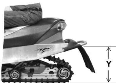
To determine sag, commonly referred to as ride-in, subtract measurement Y from X ( $\text{sag} = X - Y$ ). If the measured sag is incorrect, adjust the FRA position and/or rear torsion spring preload.
