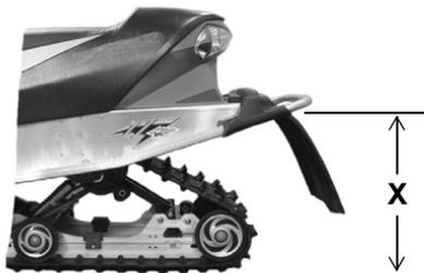
Next, have the rider drop down hard on the seat and bounce up and down several times, collapsing the rear suspension. With the rider seated, measure the distance between the ground and the rear bumper at the exact location used for measurement X. This is measurement Y.
