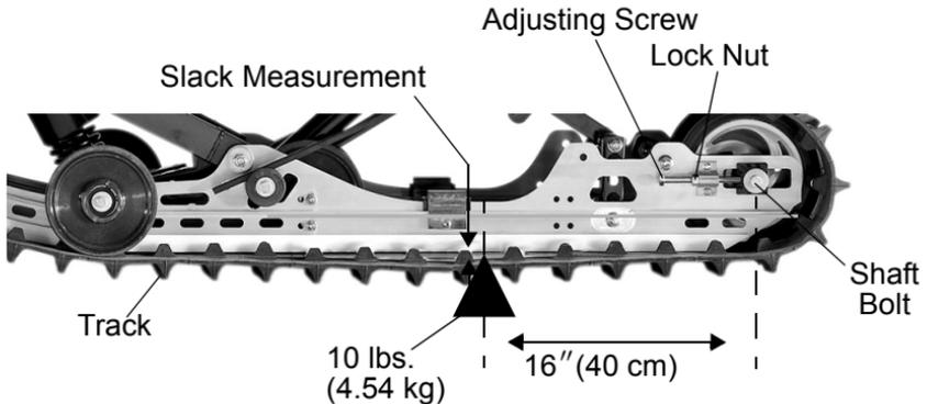
7. Tighten or loosen the track adjusting screws to provide equal adjustment on both sides of the track.
