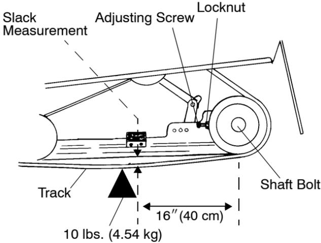
7. Tighten or loosen the track adjusting screws to provide equal adjustment on both sides of the track.
