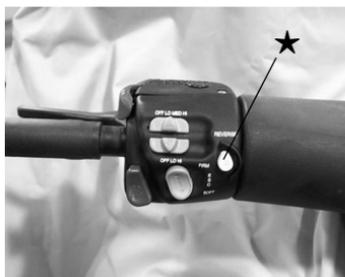
**NOTE:** The maximum engine RPM will be 6000 when in reverse.
