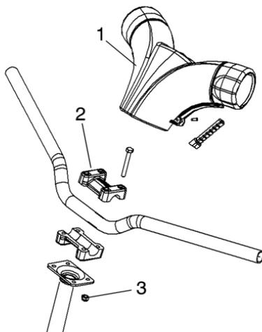
3. Adjust the handlebar to the desired height. Be sure handlebars, brake lever and throttle lever operate smoothly and do not hit the fuel tank, windshield or any other part of the machine when turned fully to the left or right.
