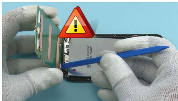
2) Place the DISPLAY to the A-COVER. Then connect the DISPLAY connector to the ENGINE BOARD. Be careful not to damage the connector.
