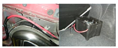
49. Battery Relocation kit is needed to move battery to back passenger side of trunk. Use supplied hardware to fasten battery cable away from moving parts, and tucked up inside frame rails as necessary. Caution! An inline fuse can be purchased separately for extra precaution when using a trunk mount battery. We recommend an inline fuse to be installed in trunk incase of fire or accidental grounding of the power cable that may cause a fire.
