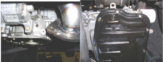
26. Using a sharp razor, carefully scrape off any silicone on the mating flange on the engine block.
