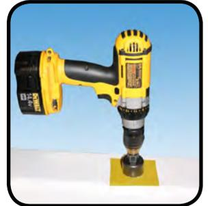
Step 3 Using a 1 ¼” hole saw, proceed to drill the large hole. Keep drill speed on the slowest speed and use lubricating oil or liquid soap to keep the hole saw cool during cutting.
