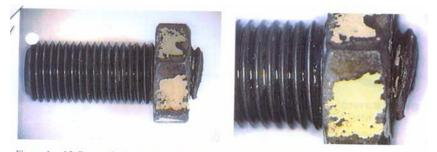
Figures 1 and 2 Fractured rod end. Note bending, through approximately 10°, associated with fracture.
