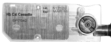
Fig. 1-19 tHb Calibration Cassette
