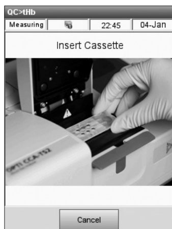
Fig. 2-19 Wipe and Insert Cassette
