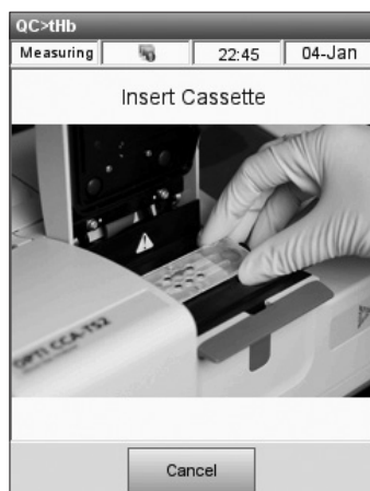
Fig. 7-8 Wipe and Insert Cassette
