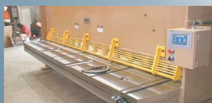
AS375-10 shown with optional ball transfers, t-slot across front edge of table and protractor
