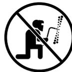
To avoid damage to the tooling, do not weld on the components. Do not modify the K-Line Jack Stands in any way by welding, heating with a torch, drilling, machining, or grinding.
