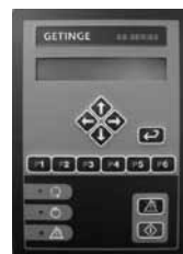
OPERATING PANEL ON SOIL SIDE
