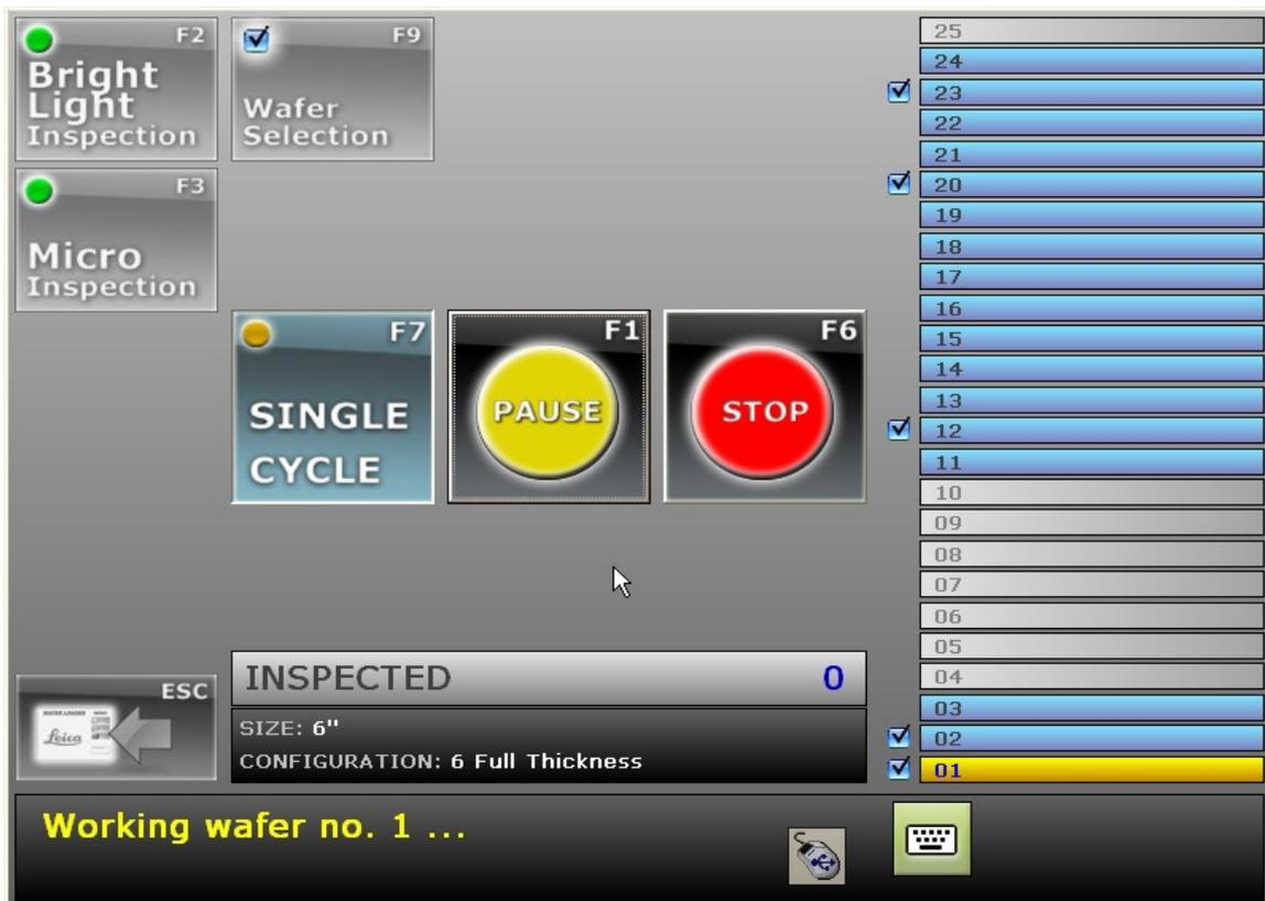
To load the first selected wafer, put the microscope stage in exchange position (left rear with the XY stage, activating the exchange sensor for at least 2 seconds) and then loader will proceed extracting the first wafer selected starting from cassette bottom.
