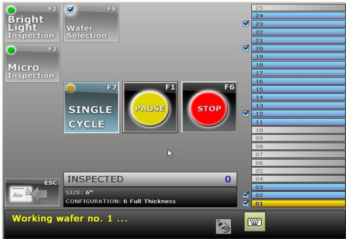
Pressing PAUSE during operation forces machine to stop at the end of the current phase or movement... It is important to remember that this key is not an instant stop key. The current movement is anyway finished and then machine stops. The next screen shows the Pause condition.
