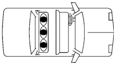
In order to use the system, you need either a forward-facing child restraint that has attaching points (B) at its base and a top tether anchor (C), or a rear-facing child restraint that has attaching points (B), as shown here.
