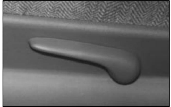
Lift the lever located on the outboard side of the seat to release the seatback, then move the seatback to where you want it. Release the lever to lock the seatback into place. Pull up on the lever without pushing on the seatback and the seatback will move forward.
