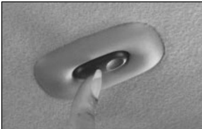
The switch works only when the ignition is on or when retained accessory power is active. See “Retained Accessory Power” in the Index.
