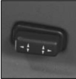
If your vehicle is equipped with this feature, the driver's and passenger's controls are located on the outboard sides of the seat cushions.
