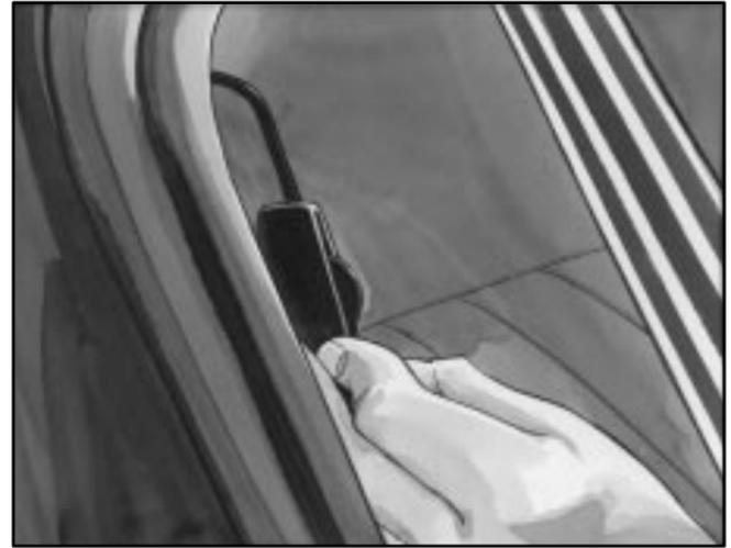
1. Pull the elastic cord out from the edge of the seatback and the interior body to remove the guide from its storage clip.
