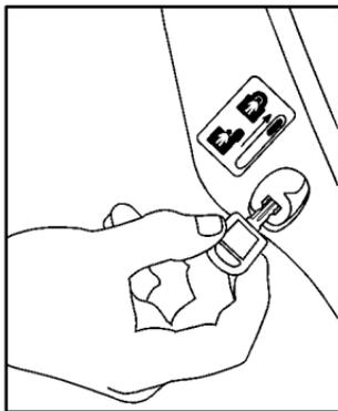
2. On the inside of the rear door will be a lock. Insert your door key into this lock and turn it upward. This will engage the safety lock. To disengage the feature, turn the lock downward.
