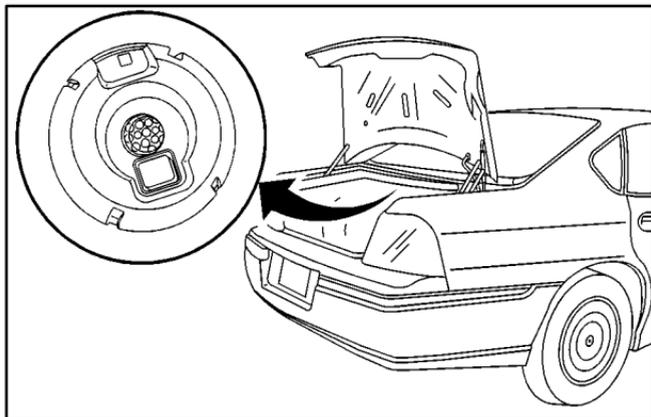
Your vehicle may have a sensor located on the underside of the filler panel inside the trunk.
