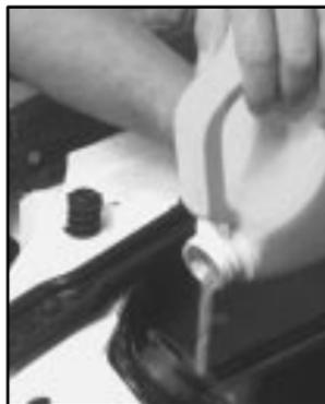
4. Fill the radiator with the proper DEX-COOL<sup>®</sup> coolant mixture, up to the base of the filler neck. See “Engine Coolant” in the Index for more information about the proper coolant mixture.
