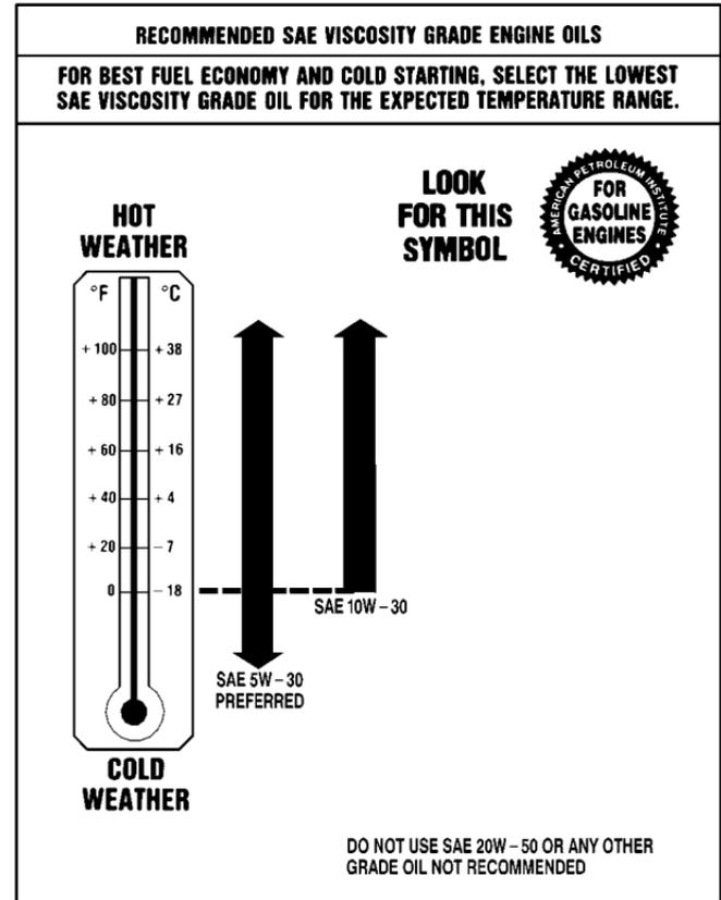
As in the chart shown previously, SAE 5W-30 is best for your vehicle. However, you can use SAE 10W-30 if it's going to be 0°F (-18°C) or above. These numbers on an oil container show its viscosity, or thickness. Do not use other viscosity oils, such as SAE 20W-50.
