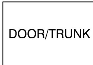
The DOOR/TRUNK light will come on if your trunk or any door is not completely closed.
