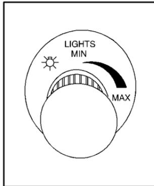
This control, located to the left of the cluster on the instrument panel, operates the exterior lamps.
