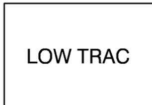
If you have the Enhanced Traction System, this light will also come on when the system is limiting wheel spin.
