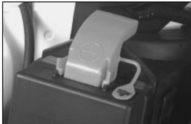
4. Open the hoods and locate the batteries. Find the positive (+) and negative (-) terminal location on each vehicle. You will not need to access your battery for jump starting. Your vehicle has a remote positive (+) jump starting terminal for that purpose. The terminal is located on the same side of the engine compartment as your battery. See "Engine Compartment Overview" in the Index for more information on location.
