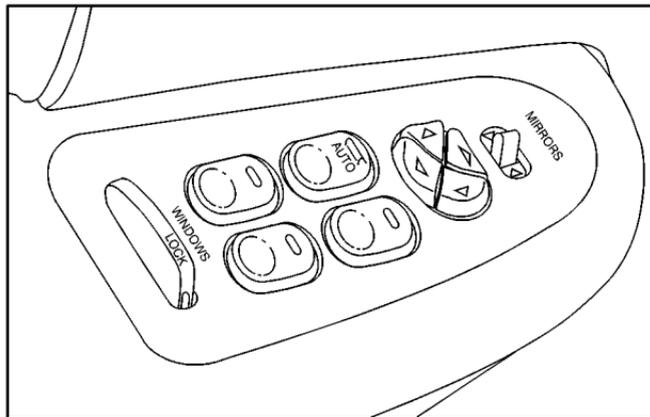
The switches on the driver's door armrest can be used to control each of the windows when the ignition is on. In addition, each passenger's door has a window switch for its own window.
