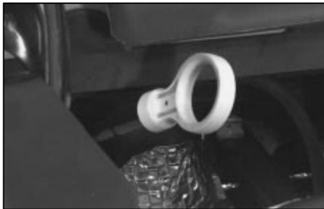
The engine oil dipstick handle is the yellow loop near the front of the engine. See “Engine Compartment Overview” in the Index for more information on location.
