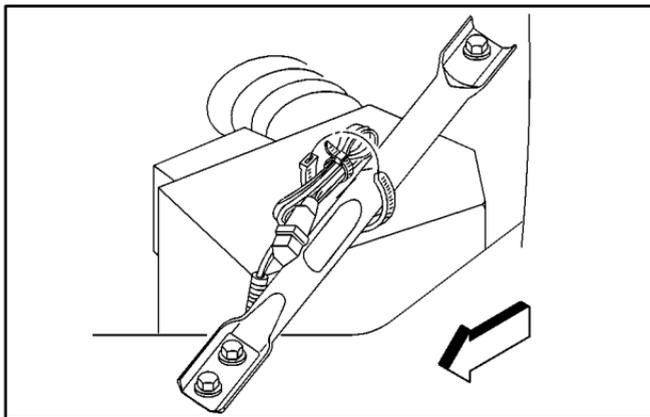
In very cold weather, 0°F (-18°C) or colder, the engine coolant heater can help. You'll get easier starting and better fuel economy during engine warm-up. Usually, the coolant heater should be plugged in a minimum of four hours prior to starting your vehicle. At temperatures above 32°F (0°C), use of the coolant heater is not required.
