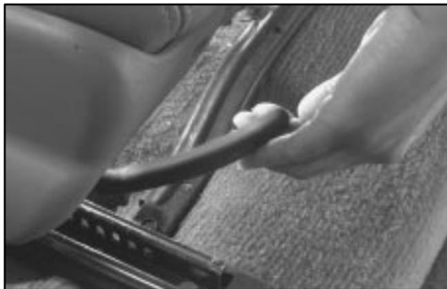
Lift the bar located under the front of the driver's and the passenger's seat. This will unlock the seat. Slide the seat to where you want it and release the bar. Try to move the seat with your body to be sure the seat is locked into place.
