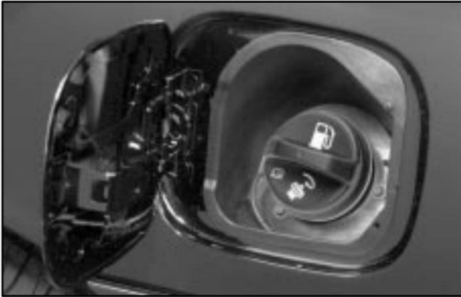
The tethered fuel cap is behind a hinged door on the driver's side of your vehicle.
