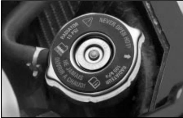
10. Then replace the pressure cap. At any time during this procedure if coolant begins to flow out of the filler neck, reinstall the pressure cap. Be sure the arrow on the pressure cap lines up like this.
