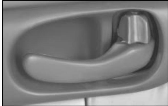
From the inside, to manually lock the door, push the lever forward. To unlock, push the lever rearward.
