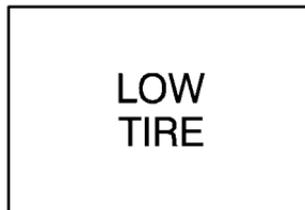
The low tire inflation monitor system can alert you to a large change in the pressure in one tire.
