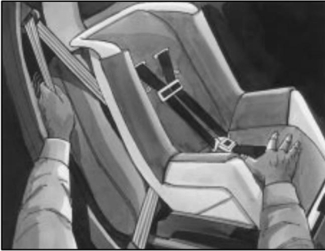
6. To tighten the belt, feed the shoulder belt back into the retractor while you push down on the child restraint. You may find it helpful to use your knee to push down on the child restraint as you tighten the belt.
