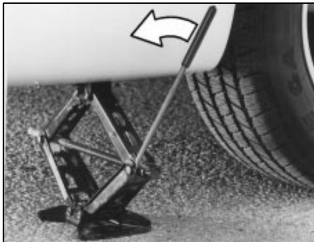
9. Lower the vehicle by turning the jack handle counterclockwise. Lower the jack completely.
