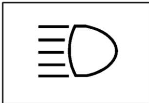
When the high beams are on this light, located on the instrument panel cluster, will also be on.
