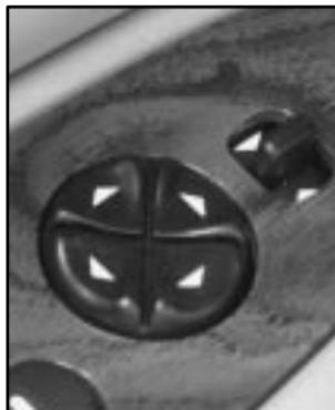
The power mirror controls are located on the driver's door armrest.
