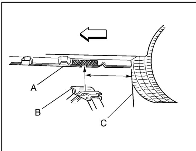
For jacking at the vehicle's rear location, put the jack lift head (B) about 5 inches (13 cm) from the front edge of the rear wheel opening (C) or just behind the off-set (A) as shown.
