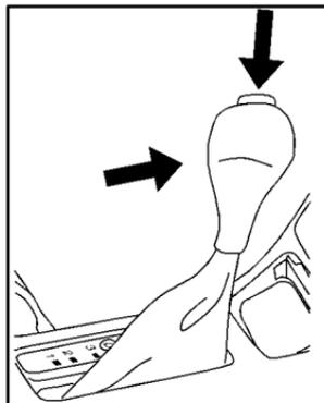
2. Move the shift lever into PARK (P) by holding in the button on the lever and then pushing the lever all the way toward the front of your vehicle. Then turn the ignition key to LOCK.
