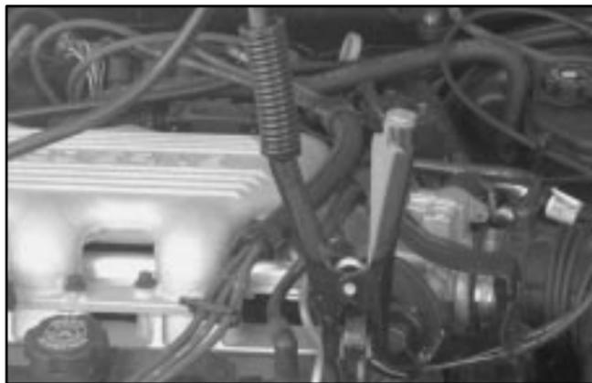
10. Now start the vehicle with the good battery and run the engine for a while.
