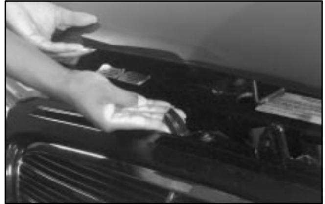
2. Then go to the front of the vehicle and release the secondary hood release by pushing it to the right.
