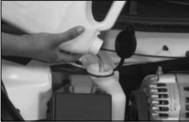
6. Then fill the coolant recovery tank to the COLD mark on the coolant recovery tank.
