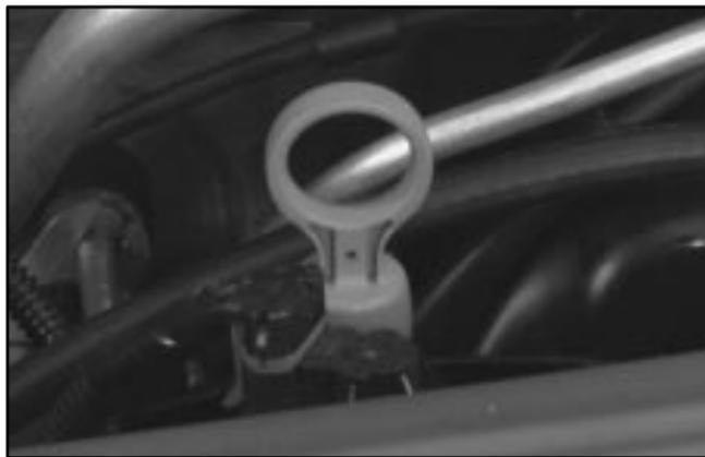
The automatic transaxle fluid dipstick handle is the red loop located toward the rear of the engine. See “Engine Compartment Overview” in the Index for more information on location.
