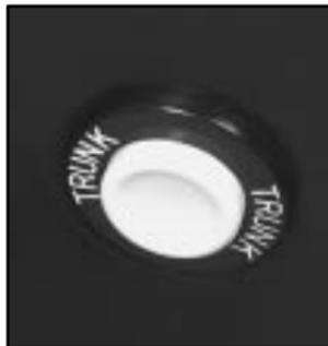
Press the button located inside of the glove box door to unlock the trunk from inside the vehicle. The shift lever must be in PARK (P) for the remote trunk release button to work.
