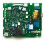
The unit has been designed for use with Atmospheric Burner gas heaters of the Intermittent Pilot type.
