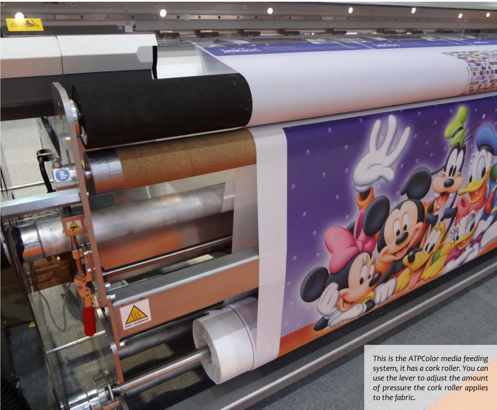
This is the ATPColor media feeding system, it has a cork roller. You can use the lever to adjust the amount of pressure the cork roller applies to the fabric.
