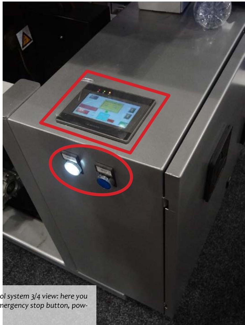
ATPColor heating unit control system 3/4 view: here you can see the touch screen, emergency stop button, power button and reset button.
