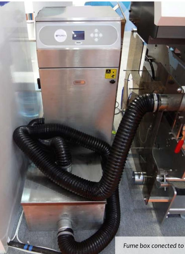
Fume box connected to the printer.
