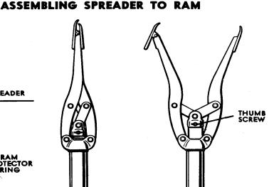
Tighten Thumb Screw on Spreader so that Spreader will retract when pressure is re-leased. Be sure to loosen thumb screw before removing Spreader from Ram.
