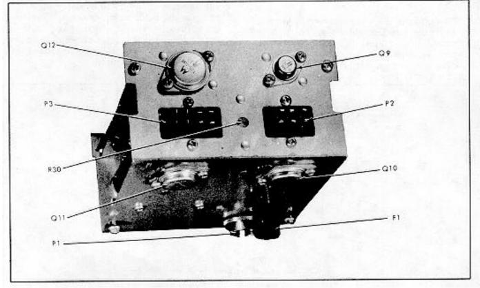
Figure 4. Rear View of Electronic Siren
