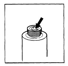
4. Check that remote actuator ring pin is properly inserted and that visual inspection seal is intact.
