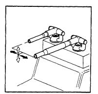
31. Quickly open and close each turret individually to check valve operation.
