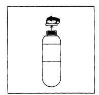
d. Screw cartridge into actuator, hand tighten.
