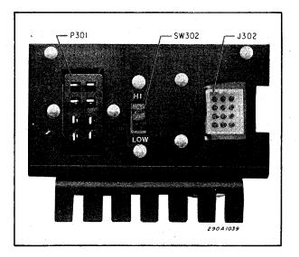
Figure 3-2. Siren Module Rear View.
