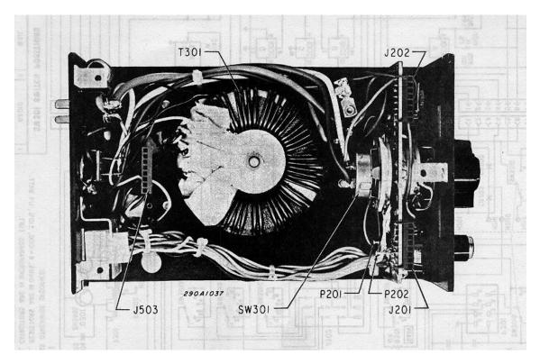
Figure 6-3. Siren Module Internal View
