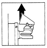
d. Screw cartridge into actuator, hand tighten.
