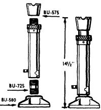
When it is necessary to operate with a broader base, add either the Flat Push Plate (BU-580) or the Cleated Push Plate (BU-581). These are connected to bottom of Ram by using the Short Nipple (BU-725).
