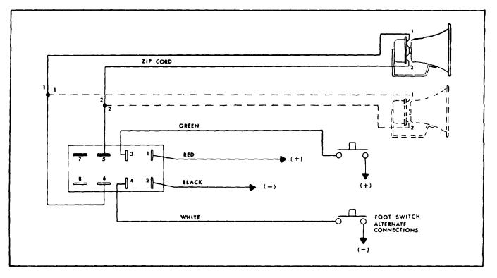
Figure 5. Power Cable Connections - Foot Switch Control
