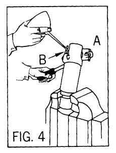
**2.** Remove filler screw A with an Allen wrench. With release valve B open, fill jack with P-F® Hydraulic Fluid using clean oil can (Fig. 5) until Hydraulic Fluid flows out of filler hole.
