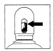
34. Secure cylinder retaining bracket(s).
