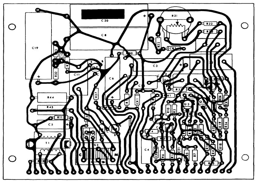
Figure 10. Component Location Diagram.
