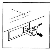
b. Remove safety shipping cap from cartridge. Weigh cartridge. Replace if weight is 1/4 ounce (7.1 9.) or more below weight stamped on cartridge.
