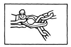
Be sure to LOCK links of Chain (BU-911) in slots of Clamp Links as shown above before starting pulling operations. For each inch of Ram travel the Chain travels TWO inches which gives longer pull without having to change the hook-up, total pull travel of 11½" without changing hook-up.
