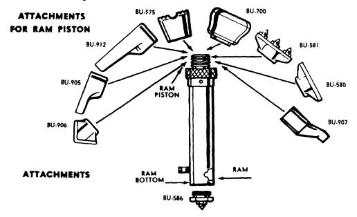
All of the above attachments may also be used on the bottom of the ram by screwing the BU-725 Short Nipple into the ram bottom.
