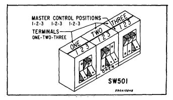
Figure 3-9. MASTER Switch Programming.
