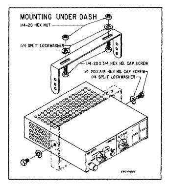
Figure 3-1. Installation of Siren Under the Dash
