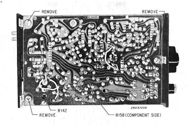
Figure 6-2. Siren Module Printed Circuit Board Removal
