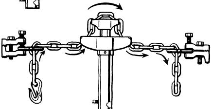
Next thread open end of Chain (BU-911) into other Bite-Tite Clamp (BU-190). Retract Ram Piston and take up slack. Lock Chain in Bite Tite Clamp Links. Close Pump Lever and start jacking operation. When Ram Piston is fully extended and further pull is required, retract Piston to same position as at start of pull, take up slack in Chain and repeat operation.
