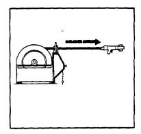
b. Open nozzle(s) fully. (Pull trigger.)
