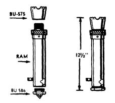
Ram can be used "as is" with Ram Cap (BU-575) attached to Piston and Ram Base BU-586 for use in restricted areas. Retracted height  $12\frac{1}{2}$ ". Extended height 18".
