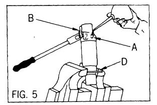
**3.** Tighten filler screw A and close release valve B. Jack ram out to full length.
