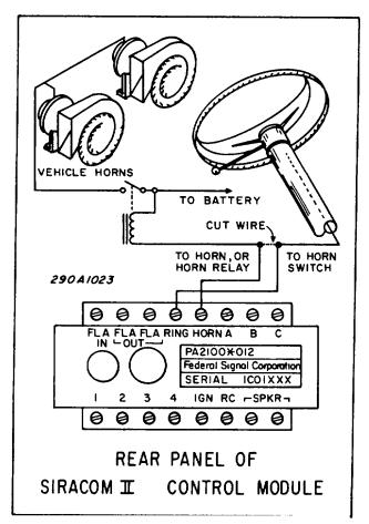
Figure 3-7. Horn Ring Connections.
