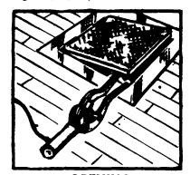
**OPENING** Spreader is being used to open metal trap door leading to basement. (Far Hook-up se(Page 17.)
