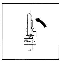
10. Pull ring pin and open GREEN Vent Valve on AFFF tank piping to relieve all remaining pressure.
