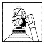
43. Seal handwheel(s) and operating lever(s) with visual inspection seals, Ansul Part No. 197.
