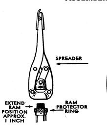
**Remove Ram Protec**tor Ring from top of ram. Extend ram piston approximately 1" and screw Spreader (BU-750) on to Ram Cylinder.
