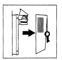
b. Remove safety shipping cap from cartridge. Weigh cartridge. Replace if weight is 1/4 ounce (7.1 g) or more below weight stamped on cartridge.
