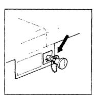
b. Remove cartridge from actuator.
