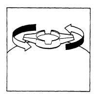
8. Make certain tank is filled with free-flowing Ansul dry chemical to a level of not more than 12 inches (305 mm) from bottom of fill opening.
