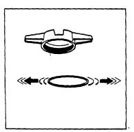
14. Check pressure relief vent in fill cap for obstruction.
