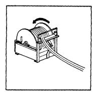
46. Secure nozzle assembly on holder and insert ring pin.
