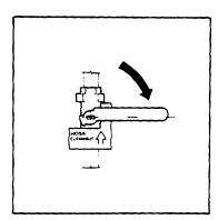
38. Secure dry chemical tank fill cap, hand tighten.
