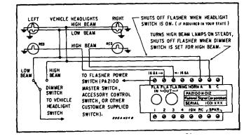
Figure 3-10. Typical Headlight Flashing circuit.
