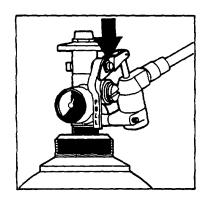
c. Insert anchor stud through valve body and actuator pivot member.
