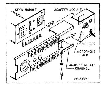
Figure 3-5. Adapter Module Installation.
