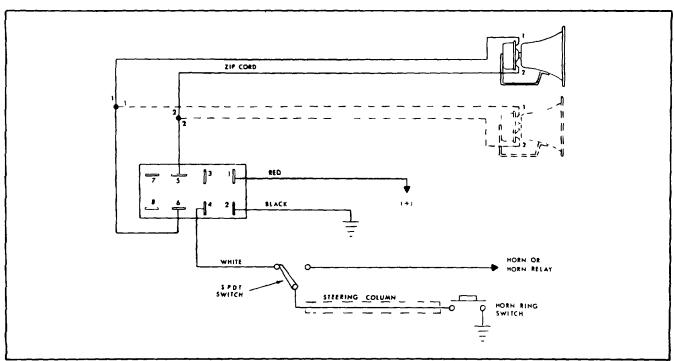
Figure 6. Power Cable Connections - Horn Ring Control (negative ground vehicles with grounded horn ring)
