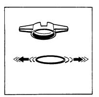
28. Clean and coat gasket lightly with a good grade of high heat resistant grease.
