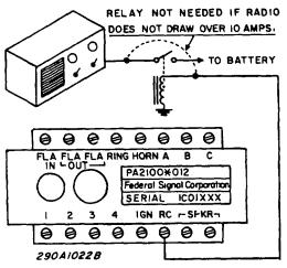
Figure 3-8. Radio Control Connections.
