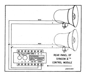
Figure 3-3. 58 Watt and 100 Watt Speaker Connections
