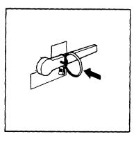
37. Insert ring pin(s) through handle(s) in bracket(s) and seal with visual inspection seal(s), Ansul Part No. 15999.
