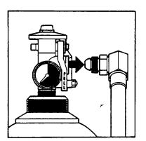
e. Thread safety plug fully into cylinder valve outlet.
