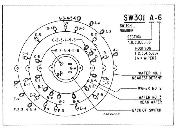
Figure 6-1. MASTER Switch Diagram
