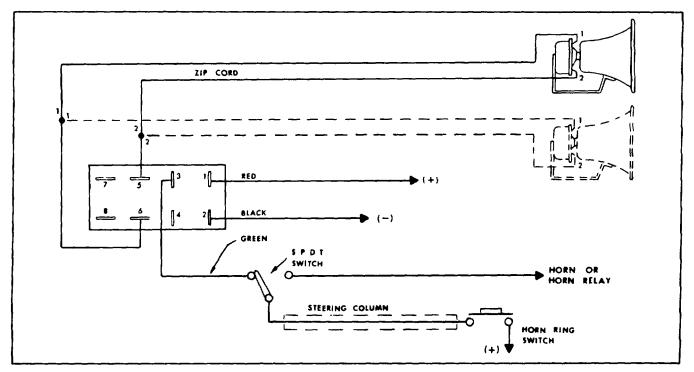
Figure 6. Power Cable Connections - Horn Ring Control (positive ground vehicles with grounded horn ring or negative ground vehicles with grounded horn ring)
