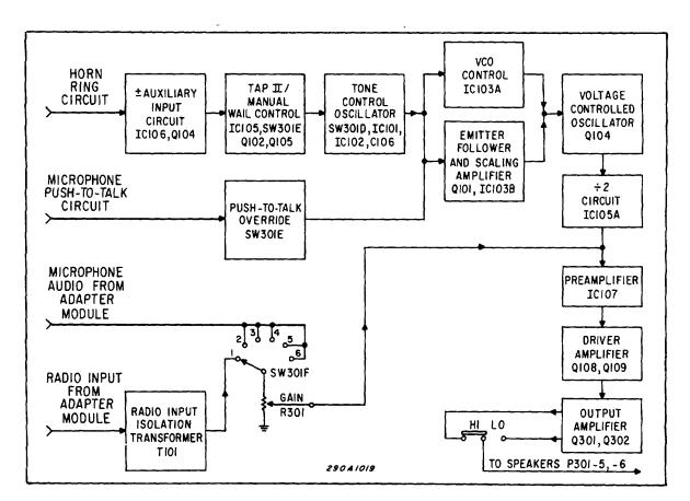
Figure 5-1. Siren Module Functional Block Diagram.
