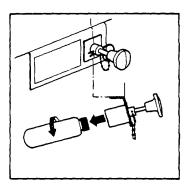
c. Remove safety shipping cap from replacement cartridge. Weigh cartridge. Replace if weight is 1/4 ounce (7.1 g.) or more below weight stamped on cartridge.
