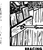
Fallen tunnel shaft being braced to allow rescue workers to speed up cave-in rescue. (For hook-up see pages 122/13,3141\$.)
