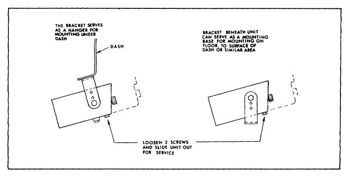
Figure 2. Positioning Unit in Mounting Bracket.
