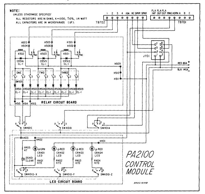
Figure 6-9. Control Module Schematic Diagram.
