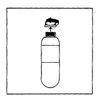
c. Raise puncture lever to assure safe cartridge installation.
