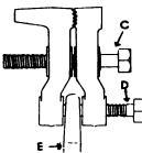
Insert Clamp Link E on Bolt D and then, holding jaws together, aw up Bolt C first ud then Bolt D.
