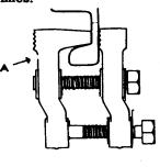
For working around channels or raised edges reverse Jaw A as shown above and proceed as above.
