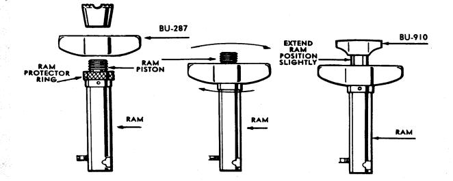
Remove Ram Cap and Ram Protector Ring from Ram Cylinder. Screw Chain Pull Collar (BU-287) on to Ram Cylinder. Be sure threaded section of center hole is next to Ram Piston. Extend Ram Piston slightly and screw Small Chain Attach. (BU-910) on to head of Ram Piston.
