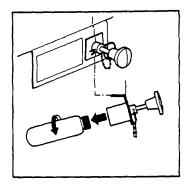
c. Weigh cartridge. Replace if weight is 1/4 ounce (7.1 g.) or more below weight stamped on cartridge.
