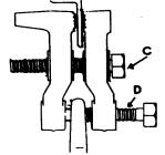
To attach Clamp to work, loosen Bolt C to provide sufficient opening for work to fit between jaws. Screw in Bolt C until Clamp is tight. CAUTION: Bolt D must remain loose. After Bolt C is tight, then screw in Bolt D to lock clamp on work. Jaws of clamps should be parallel for best holding power.
