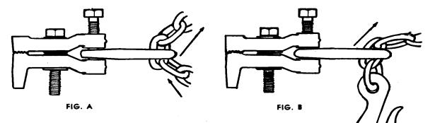
Pass small end of chain through the link hole of one of the BU-190 Bite-Tite Clamps, (Fig. A) until hookend of Chain is several inches from Clamp (Fig. B).
