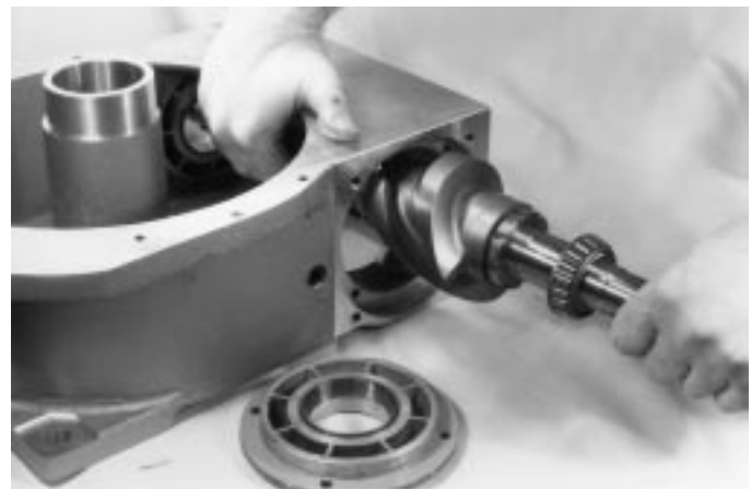
Fig. 5 Removing input shaft assembly
