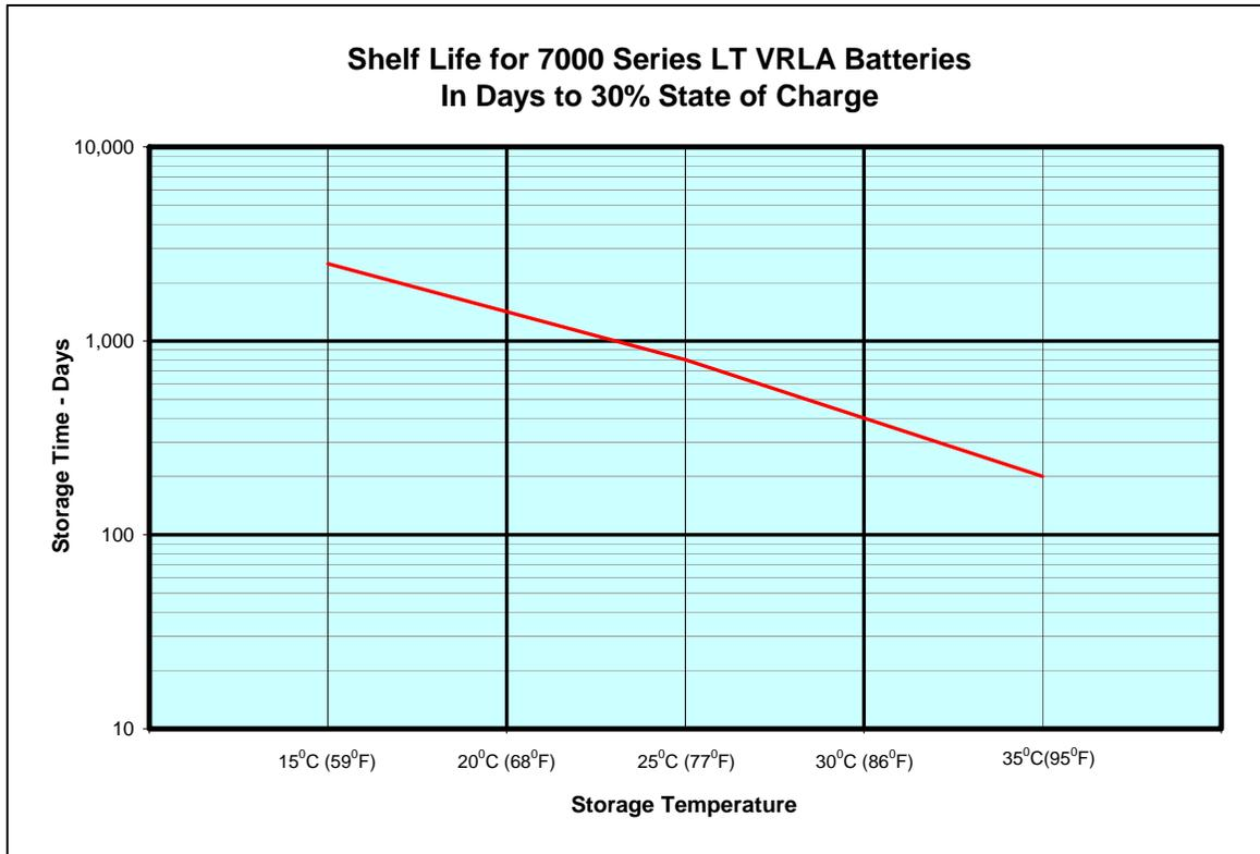
4.3.4 If stored between 95°F (35°C) to 110°F (43°C), the battery must be inspected on a monthly basis. It is not recommended to store any VRLA batteries at these temperatures for excessive periods of time (maximum 3 months storage). Prolonged storage at high temperatures (over 110°F) will reduce battery life.
