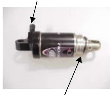
Shock in Shortest Travel Position
