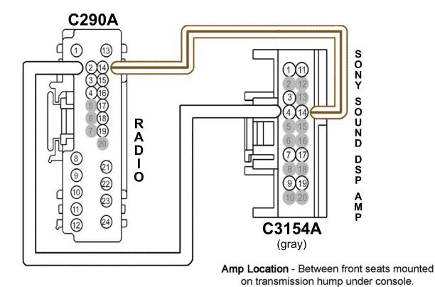
**Notes:** If the DSP already has wires in 4 & 14, cut and extend those wires from the amp to the radio. Insulate both remaining wire ends.
