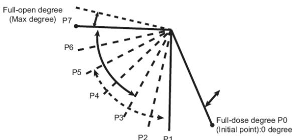
After power on, the upper and lower swing louver will automatically open and then close completely.
