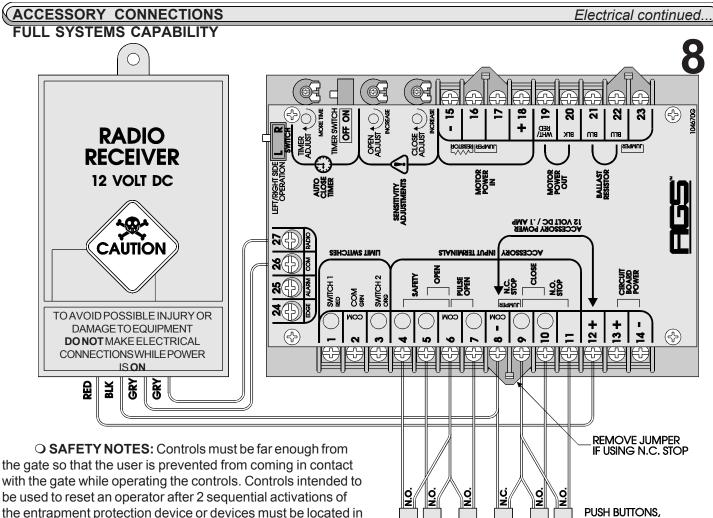
be used to reset an operator after 2 sequential activations of the entrapment protection device or devices must be located in the line of sight of the gate. Outdoor or easily accessible controls shall have a security feature to prevent unauthorized use.
