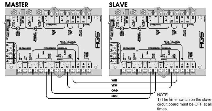
2) All peripheral devices must be connected to the master circuit board inputs.
