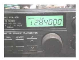
Equipment: Radio Shack HTX-100 10 Meter SSB/CW Transceiver
