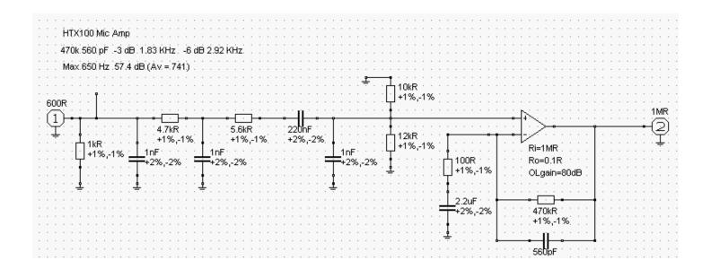
The following schematic was entered to determine the AC characteristics of the proposed improvements to the HTX-100's microphone/transmit audio amplifier; note that two resistor values and one capacitor value were changed per a chart to be found further down below.
