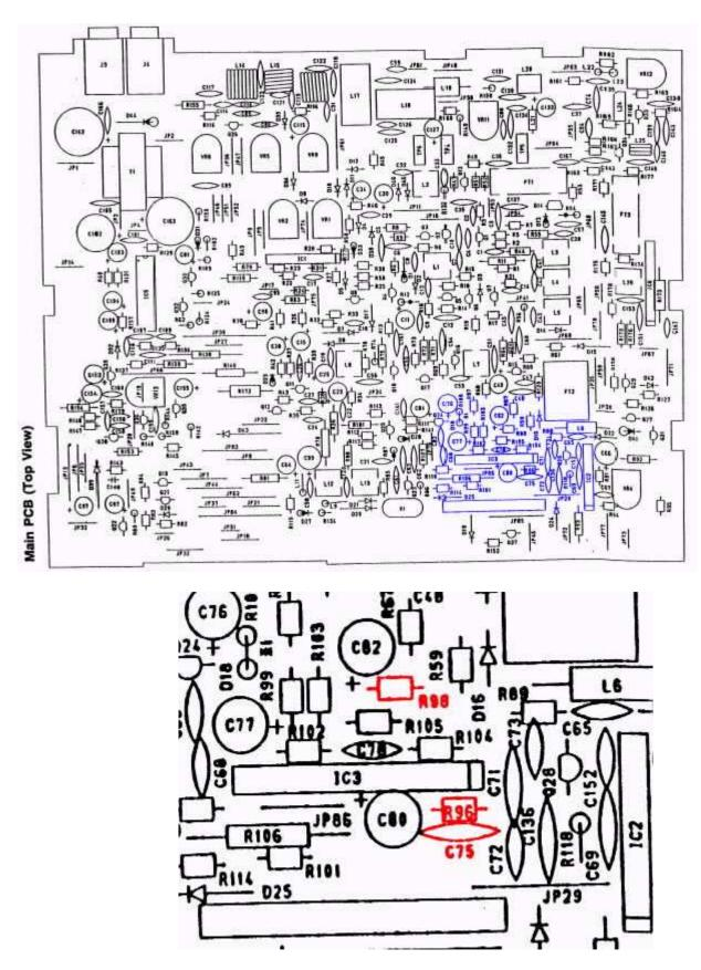
The components outlined in red are the components changed out to improve microphone amplifier frequency response. To gain access to the rear of the HTX100 Main Board and change these components the PLL
