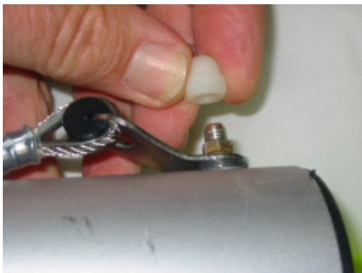
Installation of clinch nut
