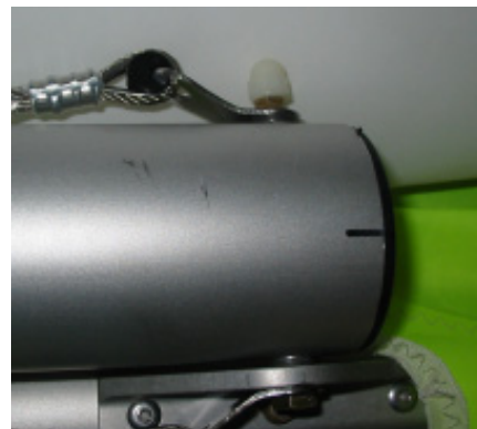
Nylon nut cap installed above clinch nut
