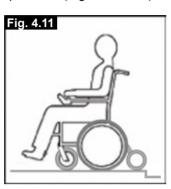
Note: In accordance to the ground clearance, the maximum obstacle height possible to climb is 5 cm (10 cm with kerb climber) for Salsa R2 and 7.5 cm for Salsa M.
