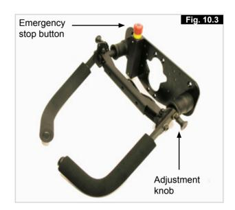
The forus push handle mechanism is centred with springs which will always bring it back to its centre position when the attendant's hands are taken off the handles. The push handles can be adjusted in height by releasing the spring loaded pin on the side, adjusting to the right height position and releasing the pin. (Fig 10.3)
