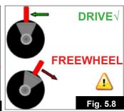
Please ensure the controller is switched off before you engage the release levers – Failure to do so will increase the force needed to push the chair.
