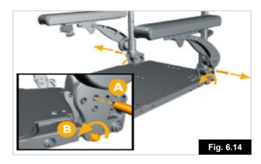
Tilt the backrest assembly forward or backward to the desired angle. See angle configurations below, (Fig.6.15 next page).
