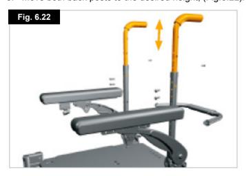
7. Replace the backpost adjustment screws. Use 10 N/m or 88.5 in/lb of torque, (Fig.6.23).
