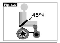
**4.32** Lap strap Rehab Seat The 5 cm (2") Aircraft Buckle lap strap. (Fig. 4.6).
