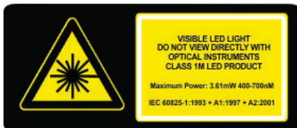
When the screen is removed, directly viewing the beam with an optical instrument (for example, an eye loop, magnifier or microscope) from a distance of less than 100mm may pose an eye hazard. MicroTiles is a class 1M source of visible and invisible LED radiation with a maximum power rating of 3.61mW @ 400-700nm.
